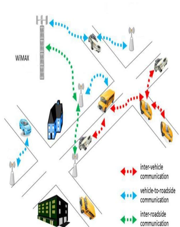
The architecture diagram describes, communication between the ITS (Intelligence Transport System) among vehicles and how to utilize DSRC and WiMAX ad hoc network in efficient ways and provide security.
