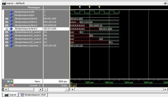
Fig. 6: Simulation Output of Tire-Pressure Monitoring Unit
