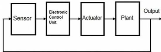
Fig. 1: Control System for a typical automobile application
