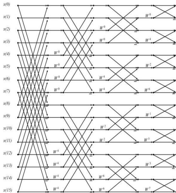
Fig. 4. Radix-2 DIT FFT signal-flow graph of length 16
