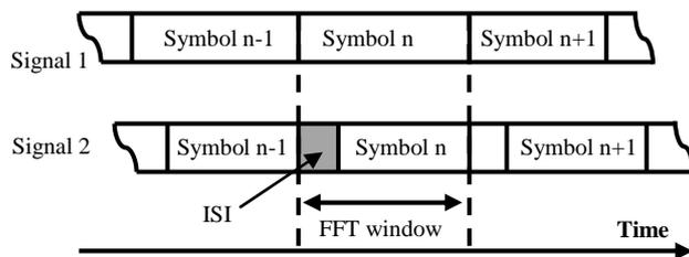
Inter-symbol interference with a delayed signal (no guard interval)
