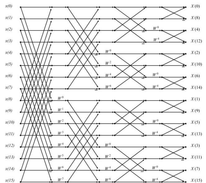
**Fig. 3.** Radix-2 DIF FFT signal-flow graph of length 16
