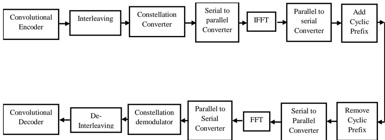
Fig. 2. OFDM Transceiver
