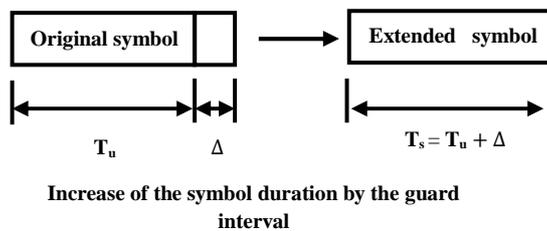
Fig. 5. ISI (Intersymbol Interference) signals
