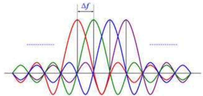
**Fig. 1.** Spectra of an OFDM sub channel an OFDM signal
