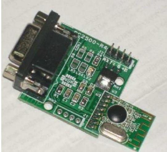
Fig 3. Zigbee Transceiver
