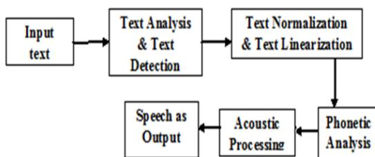
Fig. 3 Architecture of Speech Synthesizer
