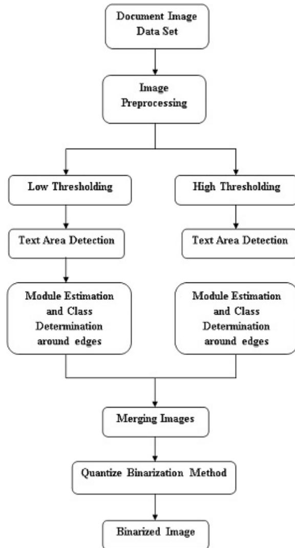
**Fig. 3. System Architecture**
