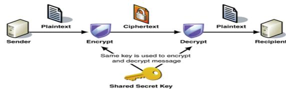
Fig 3. Symmetric Encryption
