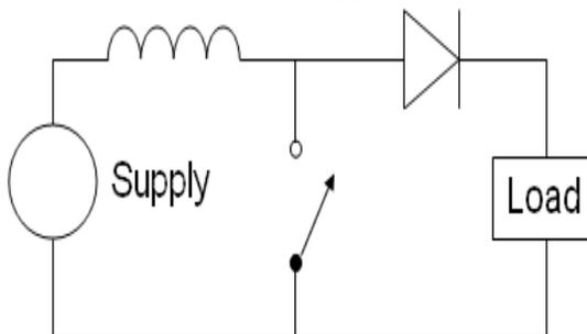
Fig: 2.2 Basic circuit of boost converter
