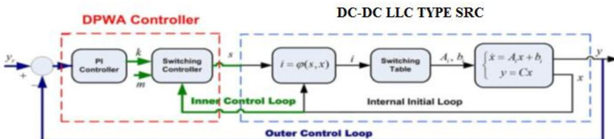
Fig. 2. Block diagram of DPWA CONTROLLER of DC-DC LLC type series resonant converter.
