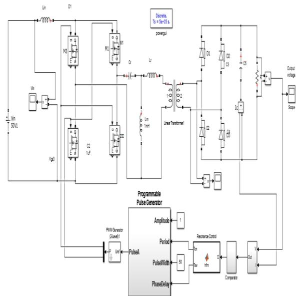
Fig 5. Simulation Diagram for dc-dc LLC type resonant converter
