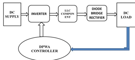
Fig. 1. Block diagram of DC-DC LLC type series resonant converter.
