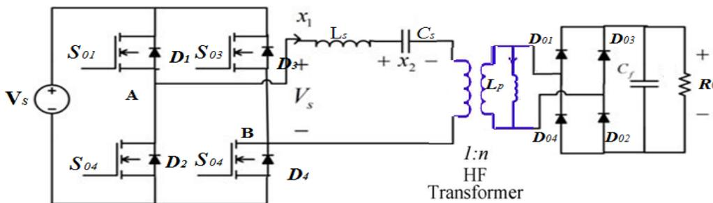
Fig.3. Circuit diagram of DC-DC LLC type resonant converter
