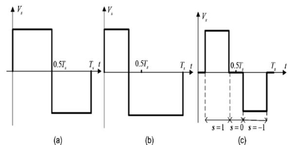
Fig. 4. Waveform of  $V_s$  for er for different control strategies: (a) frequency, (b) asymmetrical duty cycle, (c) symmetrical duty cycle
