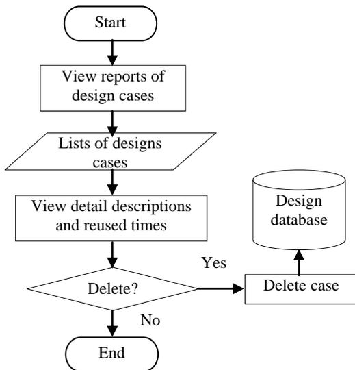
**Figure 4.** System flow for case maintenance
