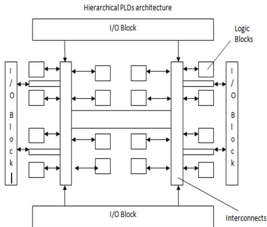
**Fig 1. FPGA ARCHITECTURE**
