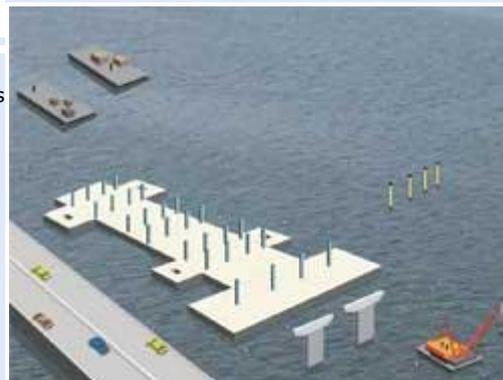
**Step 5:** Move assembled pontoons into position. Begin installation of columns on longitudinal pontoon.
