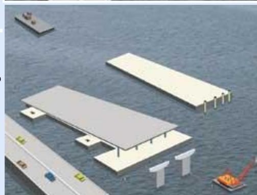
**Step 6:** Begin installation of superstructure on pontoons. Continue assembling pontoons in staging area.
