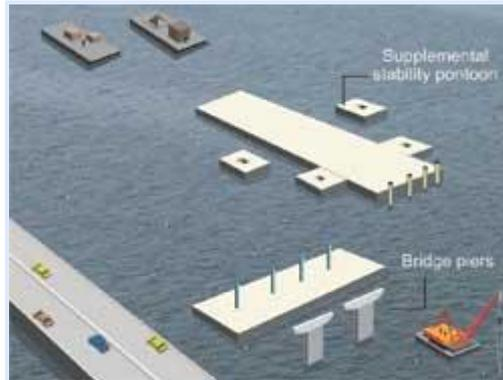
**Step 4:** Join supplemental pontoons to longitudinal pontoons at staging area. Begin installation of columns on cross pontoon.
