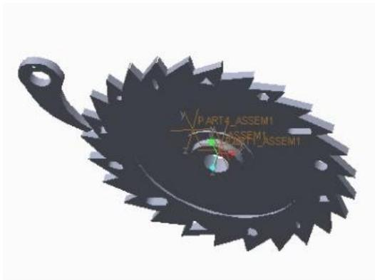
**Figure 2. Three dimensional model of Ratchet & Pawl Mechanism.**
