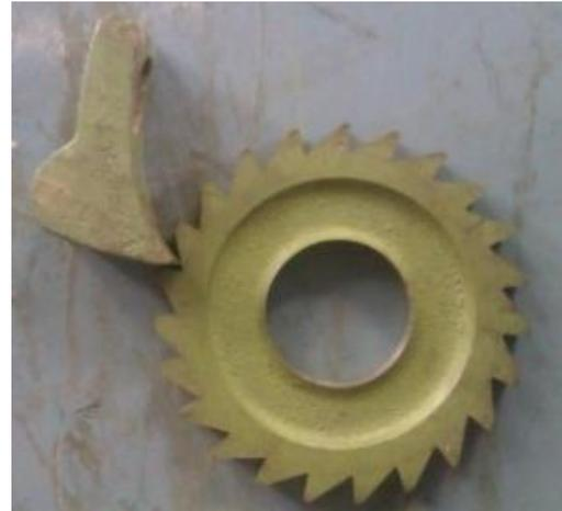
**Figure 3: Fabricated Ratchet and Pawl Mechanism**
