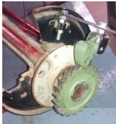
**Figure 4: Anti Roll Back Mechanism**
