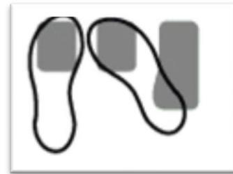
**Figure 1: Schematic representation of operating the brake, clutch and accelerator simultaneously**
