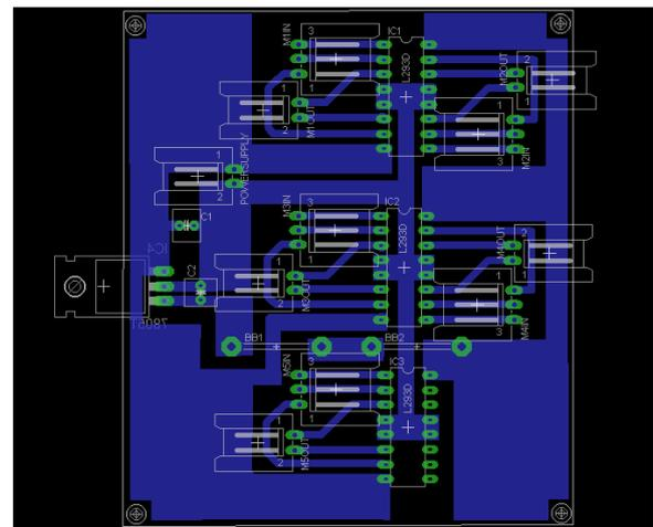
Figure 4 : Triple L293 Driver Board
