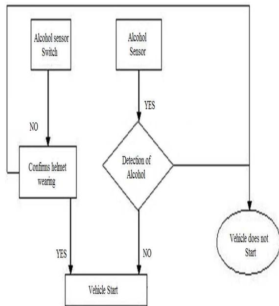
Fig 3. Flow chart of electronic smart helmet system.
