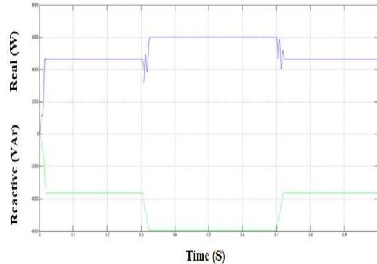
**Figure 5 Real and Reactive Power Waveform**
