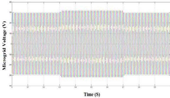
**Figure 3 Swell Voltage Waveform**
