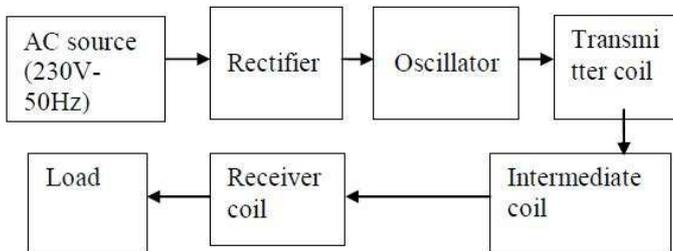
Fig 2. Block diagram representation of witricity
