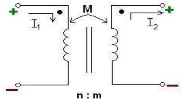
Fig 3. Transmitter and Receiver coil
