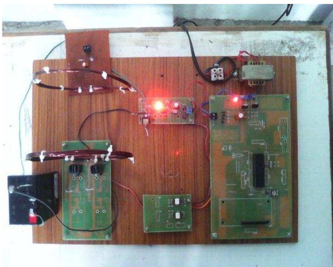
Fig 5.Hardware model for inductive coupling
