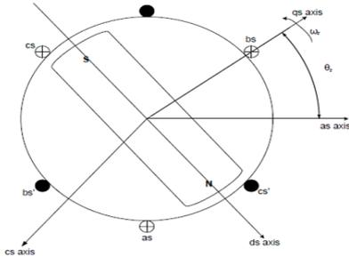
Fig 2. Two-Pose Three-Phase PMSM
