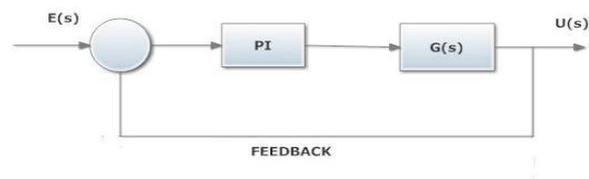
Fig 7. Block Diagram for PI Controller
