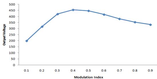
Fig.13. Inverter output voltage
