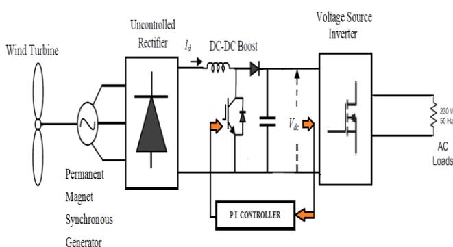
Fig.1. Block diagram for wind energy conversion
