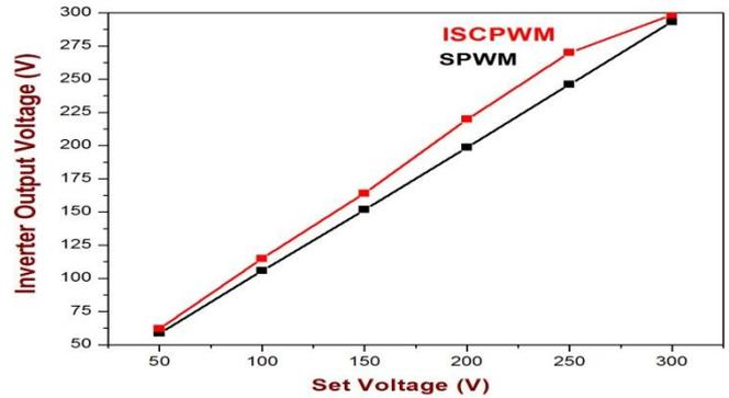
Fig.25 Inverter Output Voltage Vs Set Voltage
