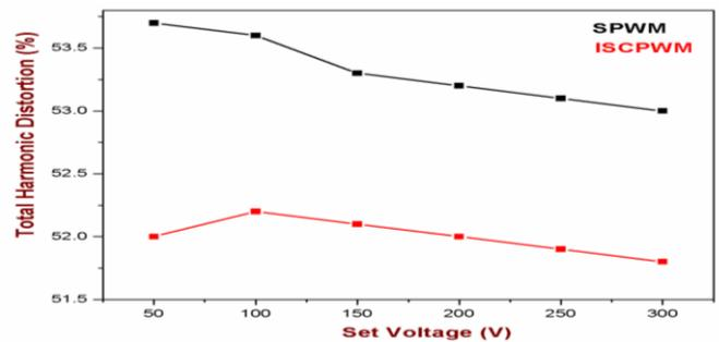
Fig.26. Total Harmonic Distortion Vs Set Voltage
