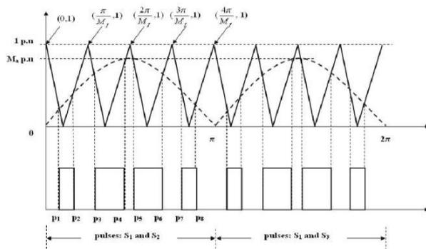
Fig. 5 .SPWM pulse generation and pattern
