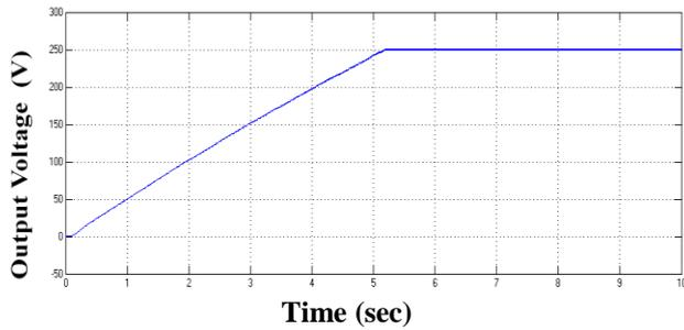
Fig.23. Boost rectifier output voltage
