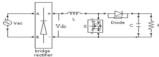
Fig. 3 .Basic boost converter
