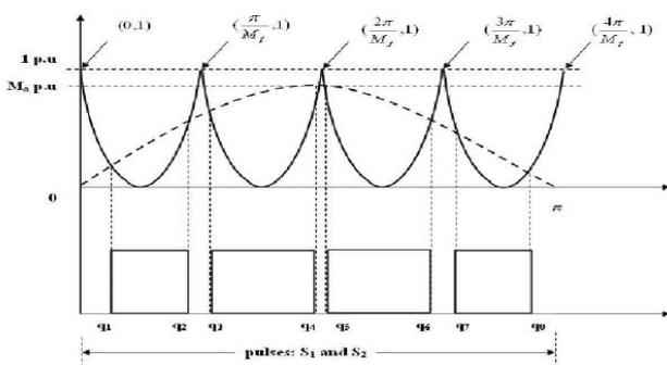
Fig.6.Inverter sine carrier PWM pulse pattern
