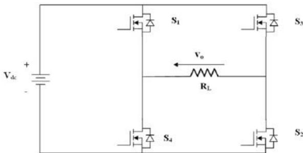
Fig.4. basic single phase e inverter
