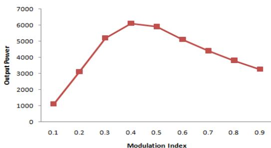
Fig.14. Inverter output power
