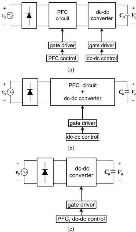
Fig 1. Block diagrams of the conventional PFC converters and the proposed converter. (a) Two-stage converter. (b) Single-stage converter. (c) Single powerconversion converter.
