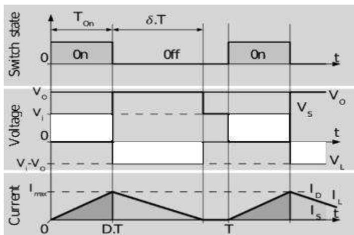
Fig 3 Waveforms of current and voltage operating in discontinuous mode.
