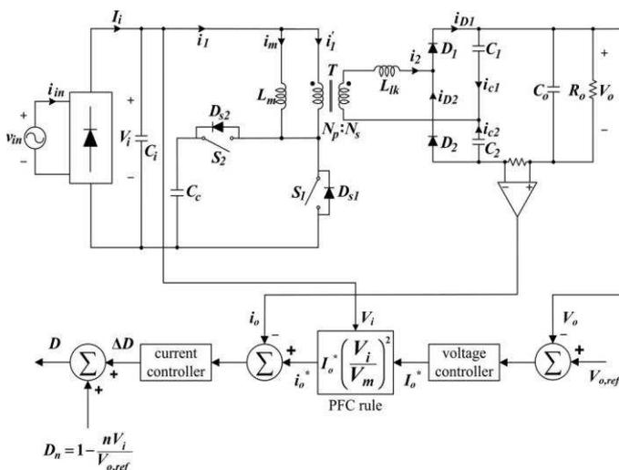
Fig 2 Proposed single power-conversion ac–dc converter and the control block diagram.
