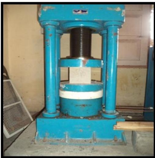
Fig: 2 Compressive strength test set up
