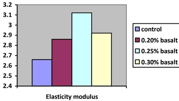
The Experimental test results shows that the cylinders made with basalt fibre concrete exhibits better Elasticity than the cylinders made with normal concrete
