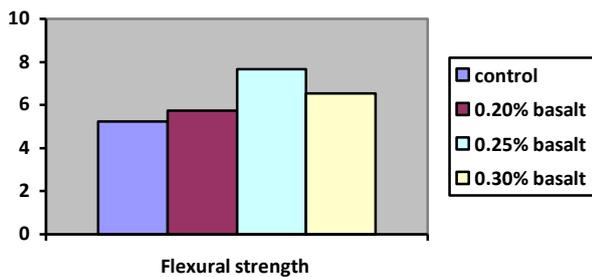
The Flexural test results shows that the Flexural strength of Basalt fibre concrete gives more strength than that of the control concrete and with 0.25% of fibre content, the strength is increased up to 40% at its optimum level and decreased gradually at 0.30% fibre content.
