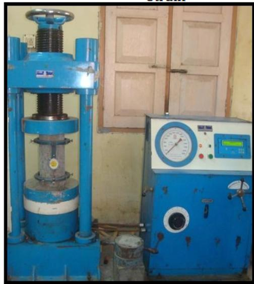
Fig: 4 Test on Concrete Cylinders for E for concrete
