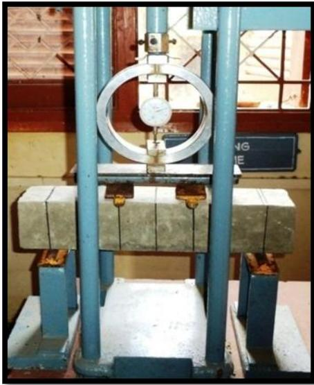
Fig: 3 Flexural strength test set up
