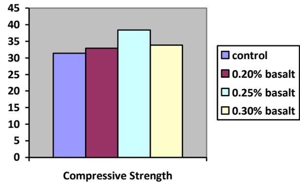
The Experimental test results shows that the compressive strength of Basalt fibre concrete is higher than that of control concrete and it is also noted that, with 0.25% fibre content the compressive strength is increased up to 25% that of control concrete and gradually decreased at 0.30% fibre content.
