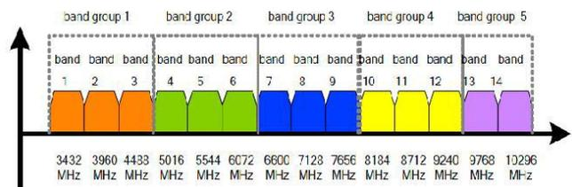
Discovering a sensible answer for maintain a strategic distance from beat related issues of drive radio (IR) UWB drives the MB-OFDM plot that consolidates OFDM tweak and multiband transmission. The MB-OFDM utilizes a 128-point backwards quick Fourier changes IFFT) and FFT with a subcarrier dividing of 4.125 Mhz (528 Mhz/128). Every information subcarrier is adjusted by a quadrature stage movement keying (QPSK) image as demonstrated in Figure
