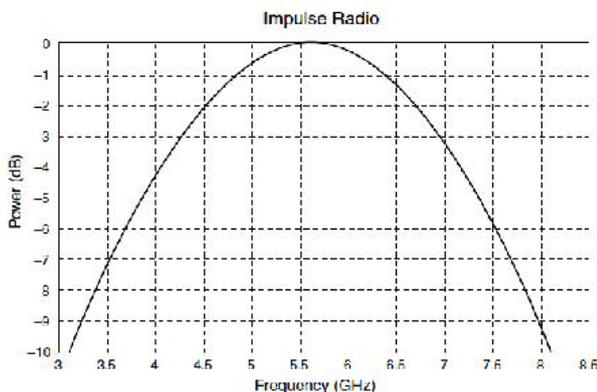
Fig2: DS-UWB transmits a single pulse over a huge swath of spectrum to represent data.
