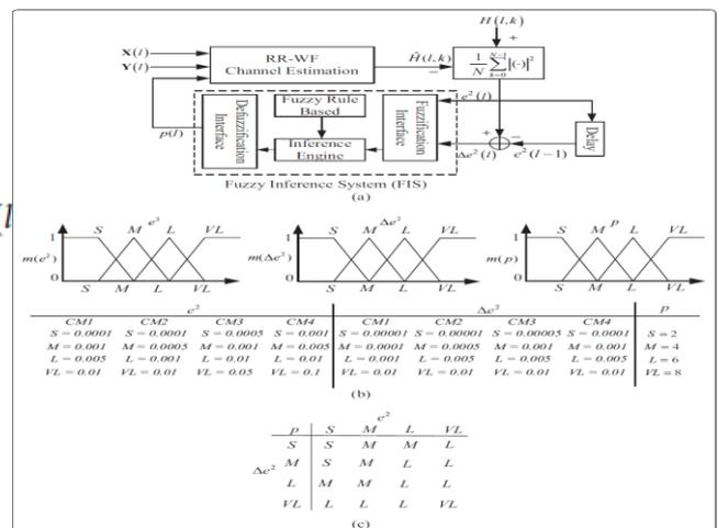
Figure 2 The fuzzy-inference-based variable filter-rank selection algorithm is illustrated by means of (a) block diagram, (b) three membership functions, and (c) predicate box, of the 2-to-1 fuzzy inference system.
