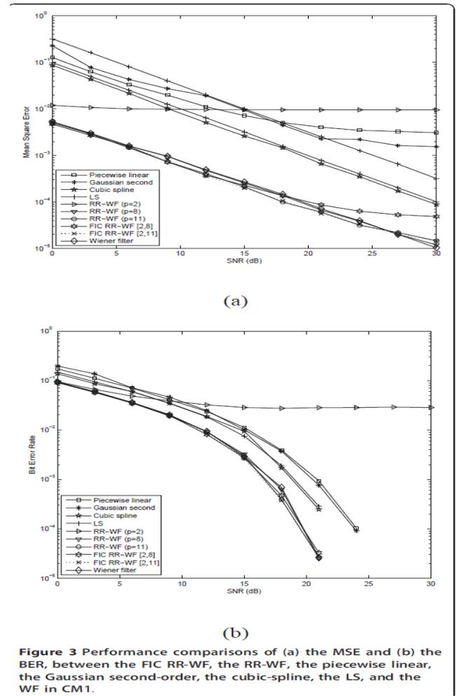
Figure 3 Performance comparisons of (a) the MSE and (b) the BER, between the FIC RR-WF, the RR-WF, the piecewise linear, the Gaussian second-order, the cubic-spline, the LS, and the WF in CM1.
