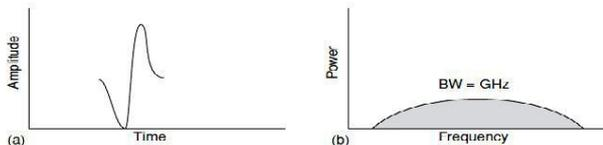
Fig: A UWB pulse in (a) the time domain and (b) the frequency domain.
