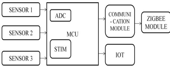
Fig 7: Block diagram of the proposed system
